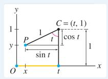
The center C of the wheel is moving rightwards at a constant speed of 1, so its position is (t,1). The angle is revolving at the same constant rate of 1 (in radians) because the radius is 1.
